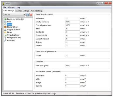
**Speed** I tend to print at 23 mm per second. The travel speed is when the printer is moving up and down to the home position.
