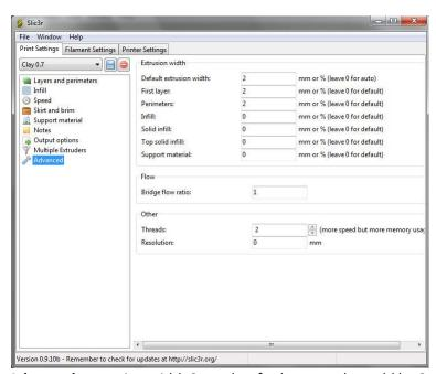
**Advanced**, extrusion width 2 mm but for larger scale could be 3 mm.
