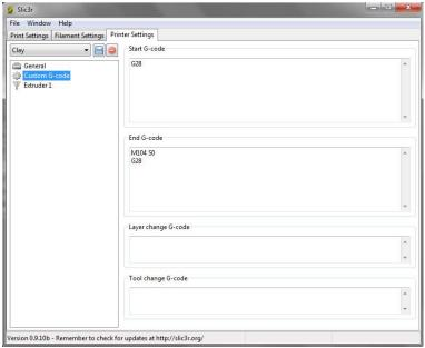
**Custom G-code**, if I remember correctly this is the default. You do want G28 in the start and end G-code. G28 is the command to go to home position that is at the endstops at the top of the printer.
