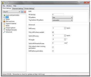
**Infill**, making hollow vessels I use 0 fill density that makes all other settings inactive. This is a setting to play with if you want internal supporting structure.
