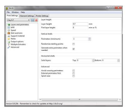
**Layers and perimeters**, this is the slice height, 0.7 is average for clay. For larger scale I go up to 0.9 and smaller scale with a smaller extruder nozzle I will go down to 0.6. Vertical shells is the number of walls to the print. I work on 1 for speed but for stability or thickness you can go 2 or 3.
